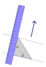
Identify the two sides of the setsquare that meet at the right angle as shown, a and b (a and bare legs of the setsquare). Place the ruler against a, and align b with one of the two lines. Notice that the ruler must be perpendicular to the line.
