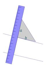
Slide the setsquare along the ruler. Try to line *b* up with the other line. If the edge of the setsquare aligns with the line, the two lines are parallel. If the edge of the setsquare does not align with the line, then the two lines are not parallel.
