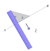
We want to draw a line through C parallel to  $\overrightarrow{AB}$ . Align b with  $\overrightarrow{AB}$ .
