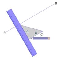
Slide the setsquare along the ruler until it is possible to draw a segment through  ${\cal C}$  along b.
